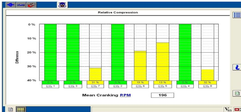
When one of the voltage peaks is 15 percent less than the others, that cylinder has low compression. If you need to know the firing order (using a labscope not the above scan tool), hook up a probe to number 1 ignition wire or coil. Do you see anything wrong with the relative compression?
