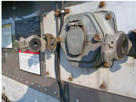
Example of wire color codes as connected to a nose box, as referenced in regulation SAE J560:
