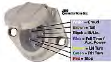
Example of wire color codes as connected to a nose box, as referenced in regulation SAE J560:
