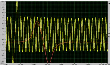
The scope is better for testing fast AC signals than the DMM. It draws each voltage pulse individually to help us distinguish between signal problems and normally occurring gaps in the signal that identify component location to the computer.
