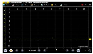
The grid is usually 10 rows high and 10 columns wide, dividing the screen into 100 blocks, called major divisions. Older labscopes were 8 rows high and 10 columns wide, dividing the screen into 80 blocks, called major divisions
