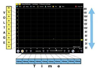
Here, we've adjusted the scope so each vertical division equals 2 volts. Since there are 10 rows on the screen, we can measure a total voltage of 20 volts at one time (10 rows x 2 volts = 20 volts).
