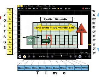
The waveform rises three divisions from the ground line. That's 3 x 2 volts = 6 volts. Our waveform has an amplitude of 6 volts.
