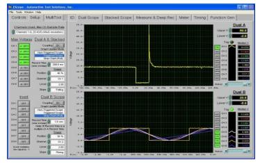
Whether it's a Big Box or a small handheld model, a "scope" is nothing more than a voltmeter that draws pictures of voltage on a screen.
