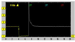
External - This is a separate scope input (commonly marked ext) that triggers the scope from an external source, regardless of the channel settings or channel voltage.
