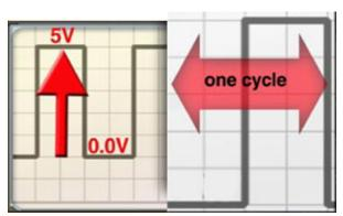
The UP and DOWN movement of the trace tells us that voltage in the circuit being tested is switching rapidly between zero and 5 volts.
