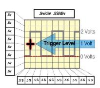
Signal Amplitude = 2 Volts
